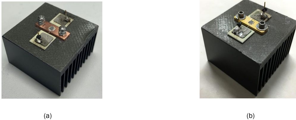
Figure I.1.20.2 (a) Preliminary power module with a single device and copper substrate, (b) Preliminary power module with a single device and metal encapsulated TPG substrate.
