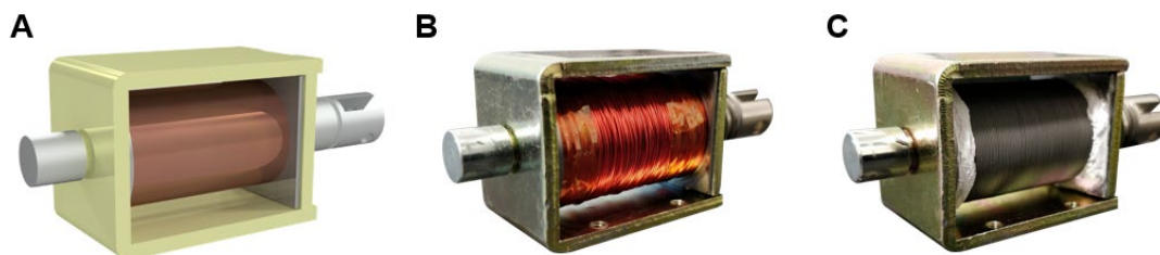
Figure I.1.21.3 A) Design, B) polyurethane prototype, and C) ceramawire prototype of the solenoid motor.
