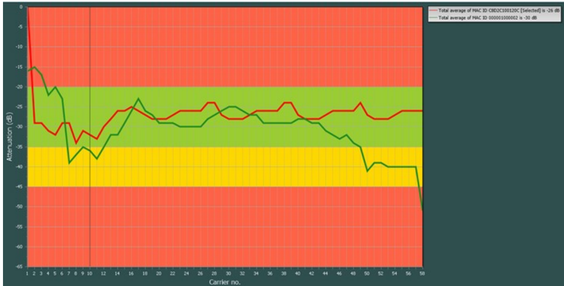
Figure II.3.1.4 BTCP 200kW - Keysight CDS PLC SLAC Attenuation
