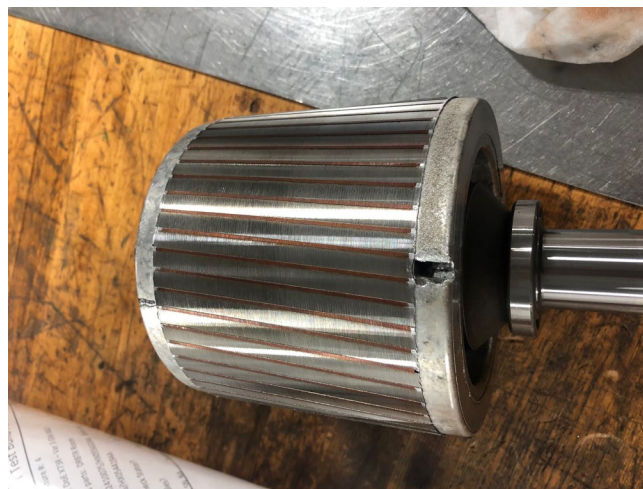
Figure I.2.6.5 Variant 3 rotor after rotor endurance failure
