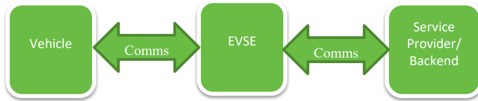
Figure II.1.20.8 Simplified EV Systems Architecture
