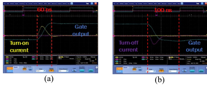
Figure I.1.26.6 (a) Zoomed-in waveforms at turn-on transient, and (b) zoomed-in waveforms at turn-off transient.
