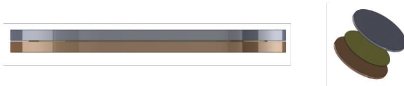
Figure I.1.9.1 Circular coupons ( \Phi 25.4\text{mm} ) for reliability evaluation; Cu (bottom) bonded to Invar (top) using sintered silver or high-lead solder (95Pb5Sn)
