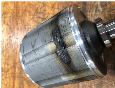
Figure I.2.6.3 Variant 2 rotor after rotor endurance failure.
