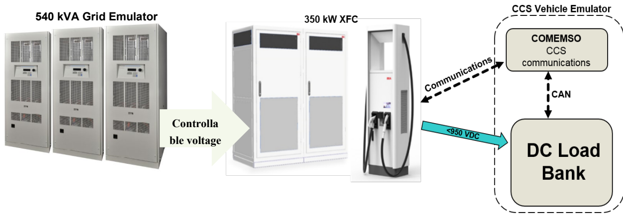
Figure II.3.3.1 Overview of high-power CCS charging emulator w/ 350kW XFC and grid emulator for variable input supply
