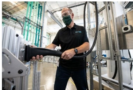
Figure II.3.4.13 Fit and ergonomics evaluation of the MCS connector and inlet at NREL
