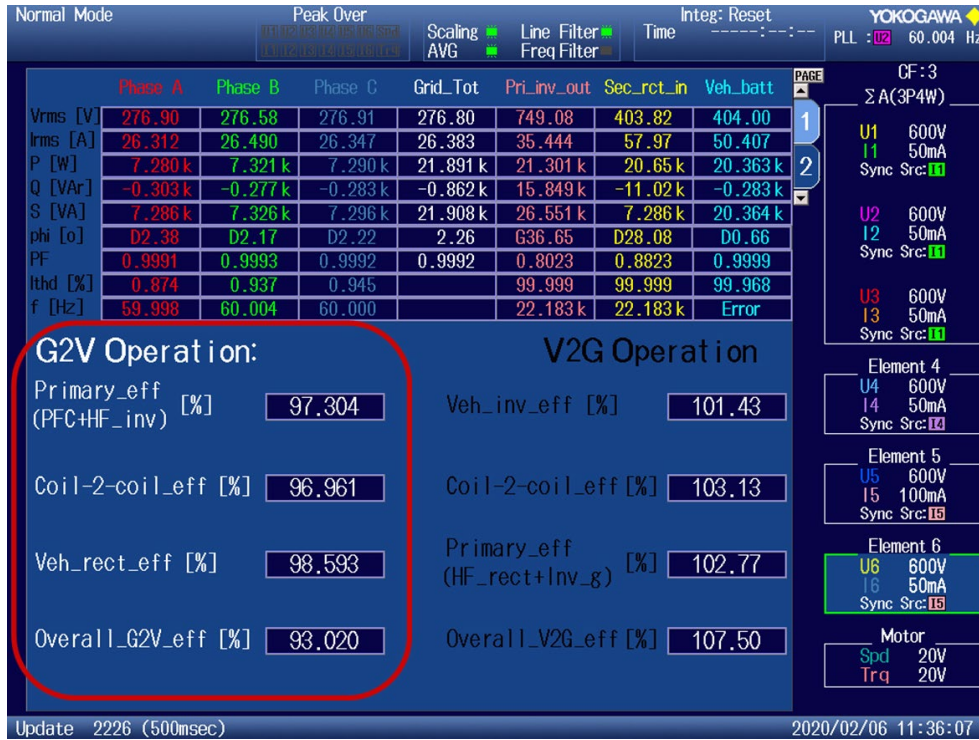
Figure II.1.15.7 G2V operation test results.
