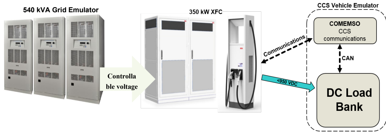
Figure II.3.3.8 Overview schematic of complete high-power charging lab research capability
