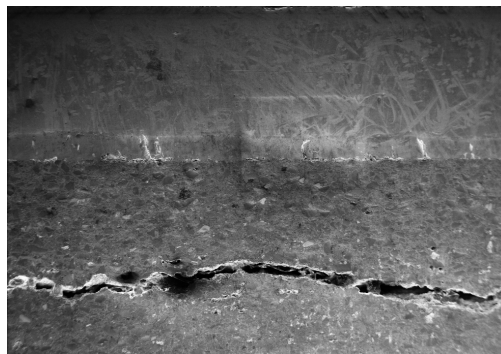
Figure I.1.25.4 SEM Image Showing crack in AlSiC
