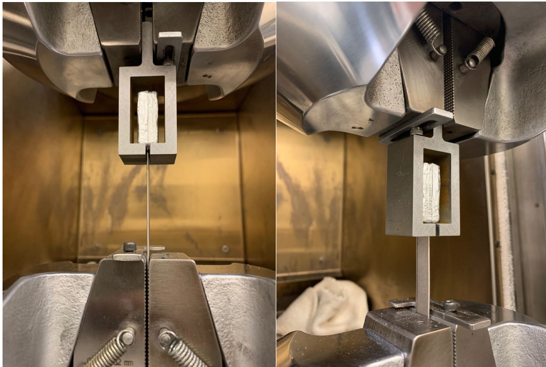
Figure I.2.6.6 Custom test fixture made for testing rotor bars.
